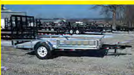
ZIMMERMAN ALUM COMBO Utility , 12x77 w/1-3,500# Axles, Rear Gate, Side ATV Ramps
