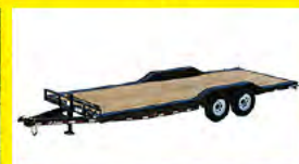
PJ B6" Channel Super Wide 20' w/2 -7K Axles 2' Dovetail 2 Standup Ramps
