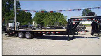
PJ FD 25' CLASSIC FLATDECK W/DUALS, TOOLBOX, 2-10K AXLES, 5' DOVE W/3 FLIPOVER RAMPS, RAMP SUPPORT ARMS
