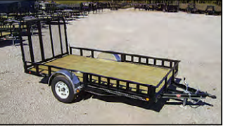
PJ U7 12'x77" CHANNEL UTILITY, 1-3,500# AXLE, STRAIGHT DECK W/4' FOLDUP GATE, SIDE ATV RAMPS, SPARE TIRE MOUNT
