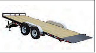
PJ TH 20'x83" HYDRAULIC QUICK TILT, 2-5,200# AXLES, SPARE TIRE MOUNT
