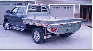
ZIMMERMAN ALUM COMBO FLATBED, W/B&W HITCH & REAR RECEIVER HITCH
