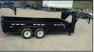
PJ DJ 16'x83" LOW PRO XL DUMP, 2-7K AXLES, SPLIT/SPREADER GATE
