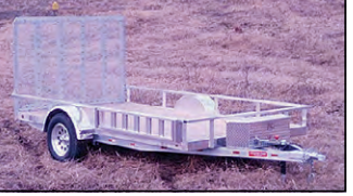
ZIMMERMAN ALUM COMBO UTILITY 12', 1-3,500# AXLE, REAR GATE, SIDE ATV RAMPS
