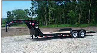
PJ T6 22'x6" CHANNEL EQUIPMENT TILT, GN, TOOLBOX, 2-7K AXLES, 16" TILT DECK
