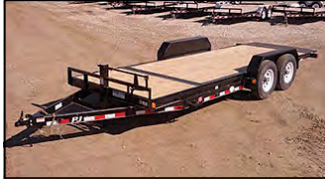
PJ T6 20'x6" CHANNEL EQUIPMENT TILT, 2-7K AXLES, 16" TILT DECK
