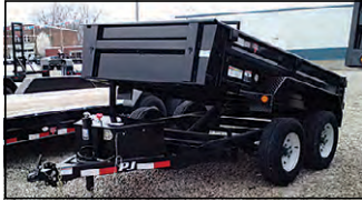
PJ D5 10'x60" UTILITY DUMP, 2-5,200# AXLES, SPLIT/SPREADER GATE
