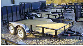
PJ U8 16'x83" CHANNEL UTILITY, 2-3,500# AXLES, STRAIGHT DECK
